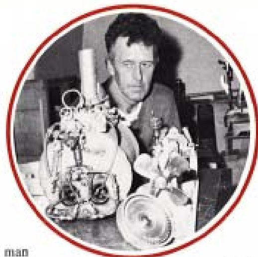
ENGINEER Ralph Watts Smith looking at his handwork. The boiler, with smoke uptake, is at the left, and the turbine and variable-pitch propeller on its shaft are at the right.
