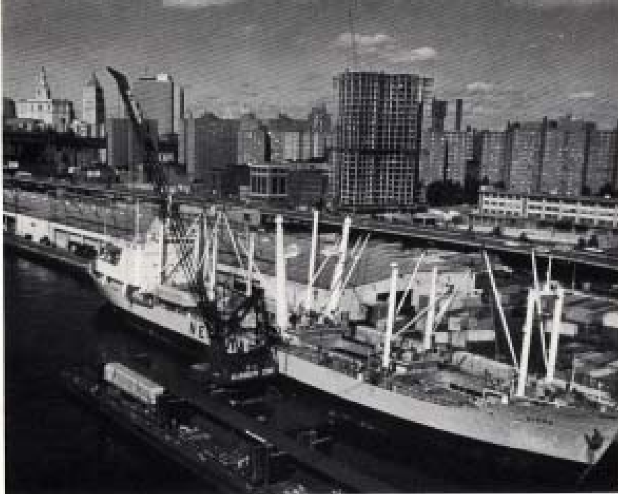
HEAVY LIFT, EAST RIVER - Bound for Brazil, six locomotives (at 156,600 lbs. ea.) are placed on deck of Netumar Line's M.V. Diana at busy Pier 36 by the M.J. Rudolph Corp. crane R-13. Tug Harriet Moran placed the R-12 earlier, after towing the fully-revolving crane from Port Newark, New Jersey.
