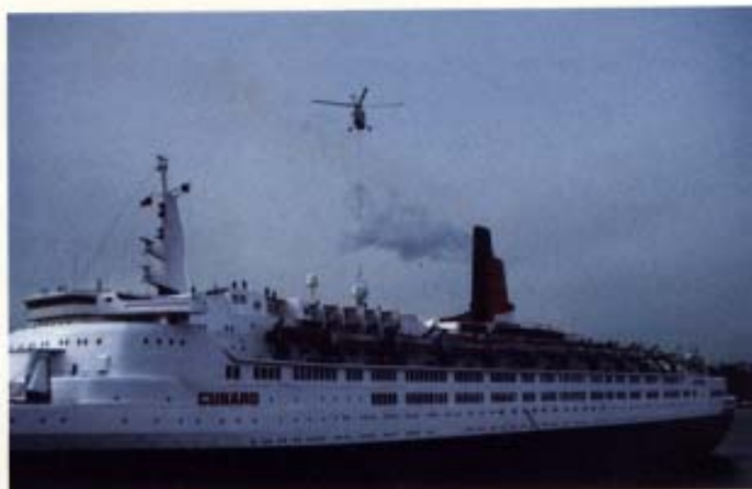
Communication Satellite Corporation (COMSAT). The radome and gyroscopic tracking mechanism package, weighing 1,100 lbs., was placed aboard the ship with a helicopter while she was in the Passenger Ship Terminal.
