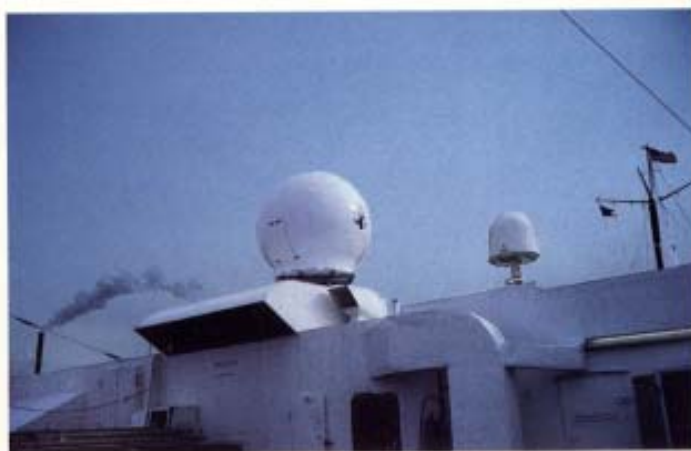
Passengers cruising off the coast of Peru on the QUEEN ELIZABETH 2 this year didn't miss Super Bowl Sunday, thanks to the installation by Cunard of a Sea Tel antenna on the ship in January, just before her world cruise, to receive live TV transmission via satellite. The test system was set up by the
