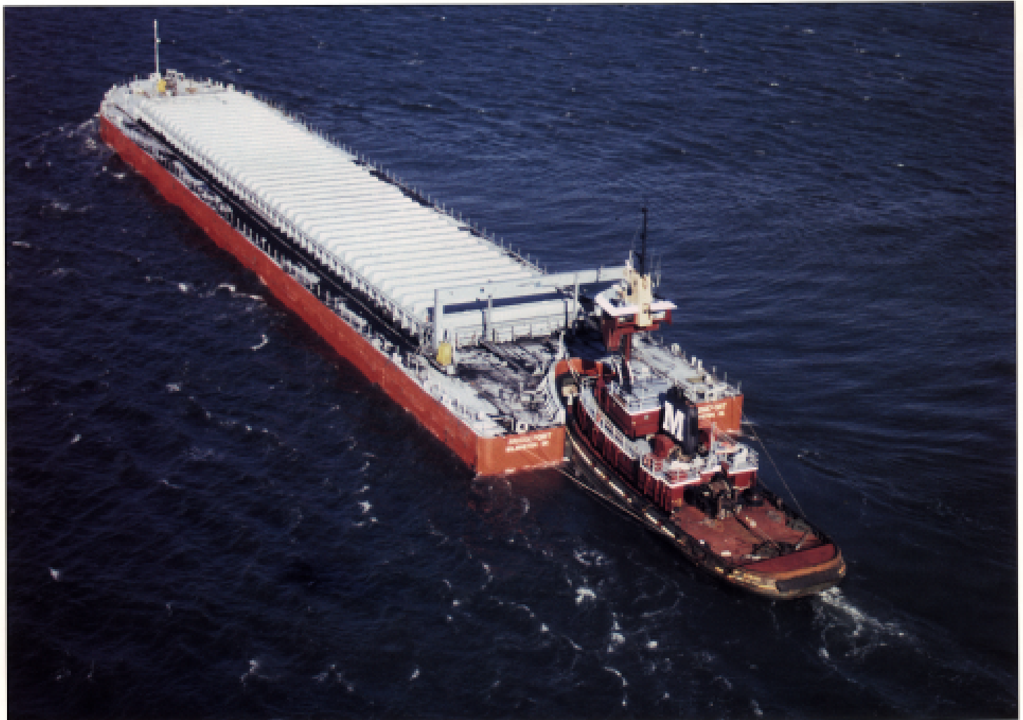
The 3,300 HP AMY MORAN pushes the 418-foot long dry bulk barge BRIDGEPORT, loaded with a cargo of coal.
