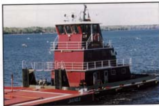
The TILLIE MORAN is one of four new 65-foot, 1,000 HP pushboats built to service the Petco contract with Florida Power & Light.
