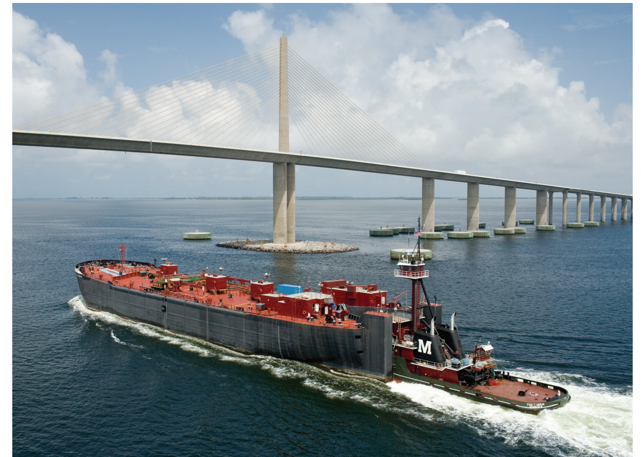
Below: The Massachusetts, a Moran double-hull petroleum barge with ATB coupling that enhances speed and maneuverability.
